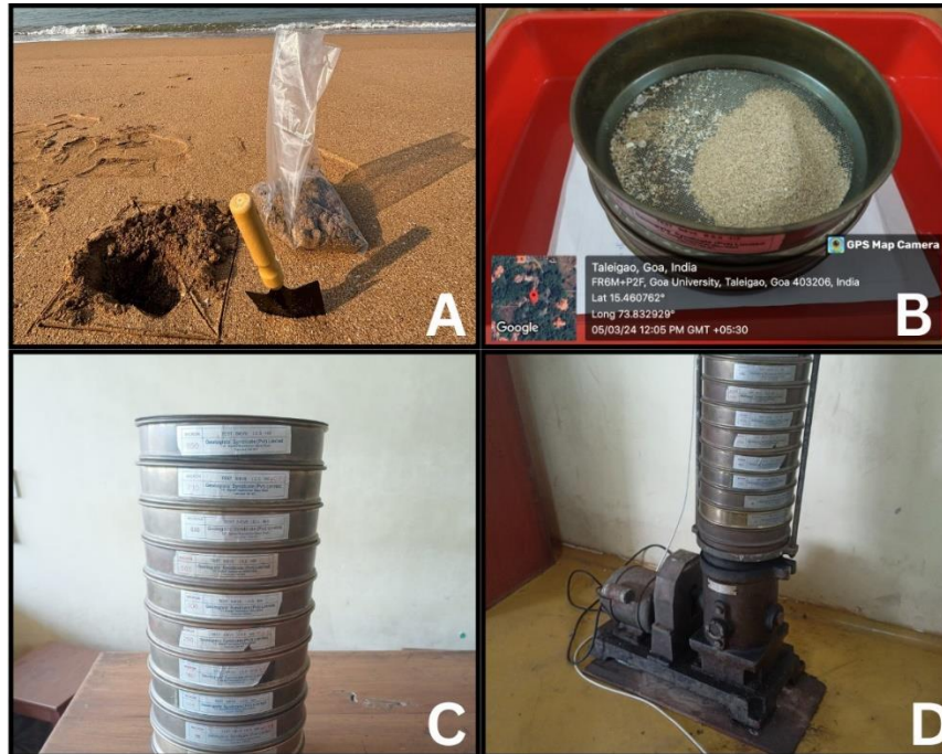
FIGURE 16 . A. sample collection. B. sample cleaning. C. arrangement of sieves. D. sieve shaker.
