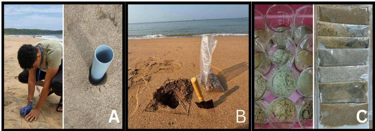
FIGURE 15 a) the core tube is pushed into the sediments with the head of the plunger remaining on the surface. b. sample collection for sieve size analysis c. sample storage.
