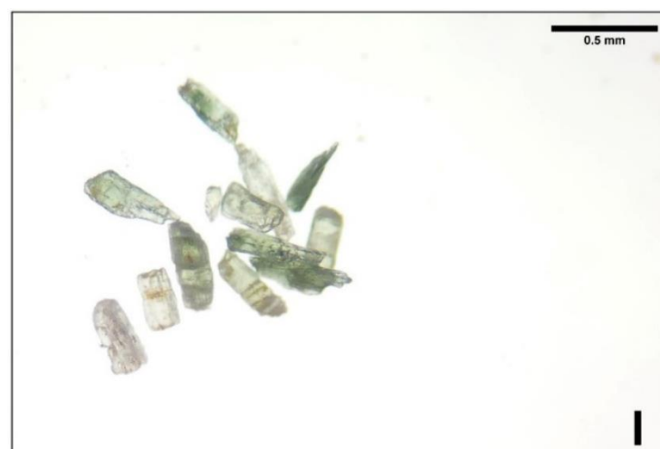
FIGURE 33 :- Tremolite Grain from Sample M5BS
