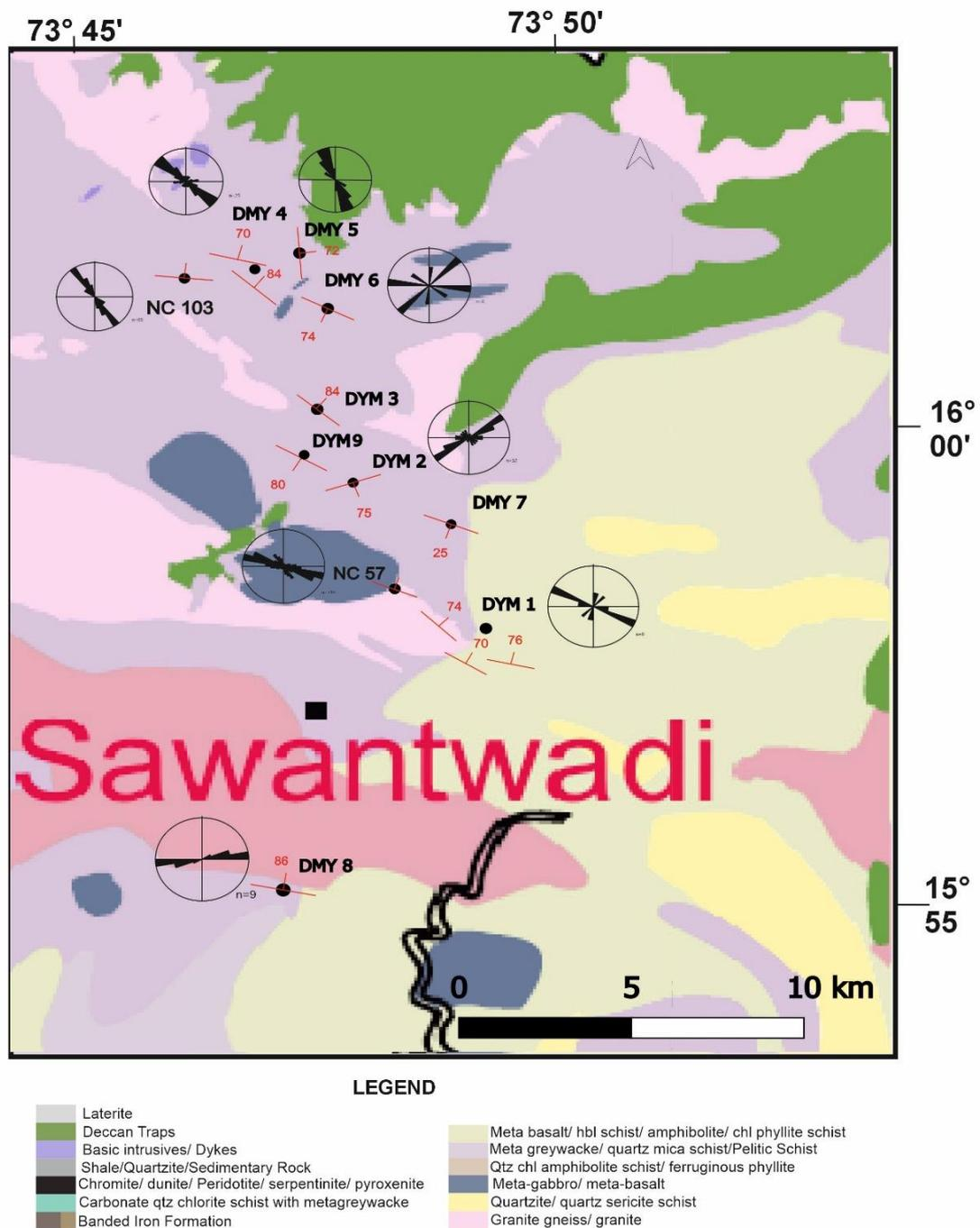
Figure 4 Lithological map of the study area modified after GSI(2021) District Resource map of Sindhudurg, Keyed to the map are penetrative foliations in each outcrop and rose diagram plots of the orientation of steep quartz veins.
