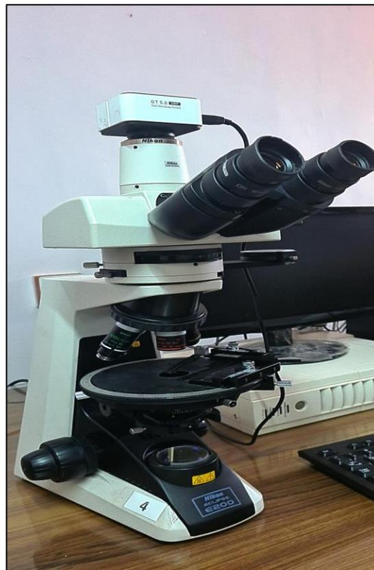
Figure No.08 : Nikon ECLIPSE E200 microscope
