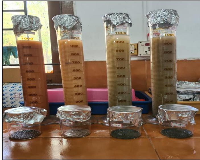
Figure No.04: Samples kept for settling in 1000 ml volumetric beakers
