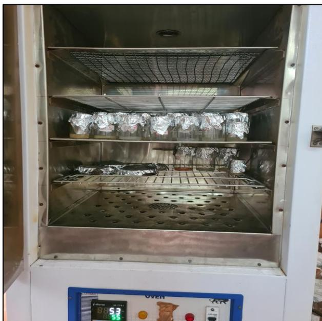
Figure No.07: Clay Samples kept for drying
