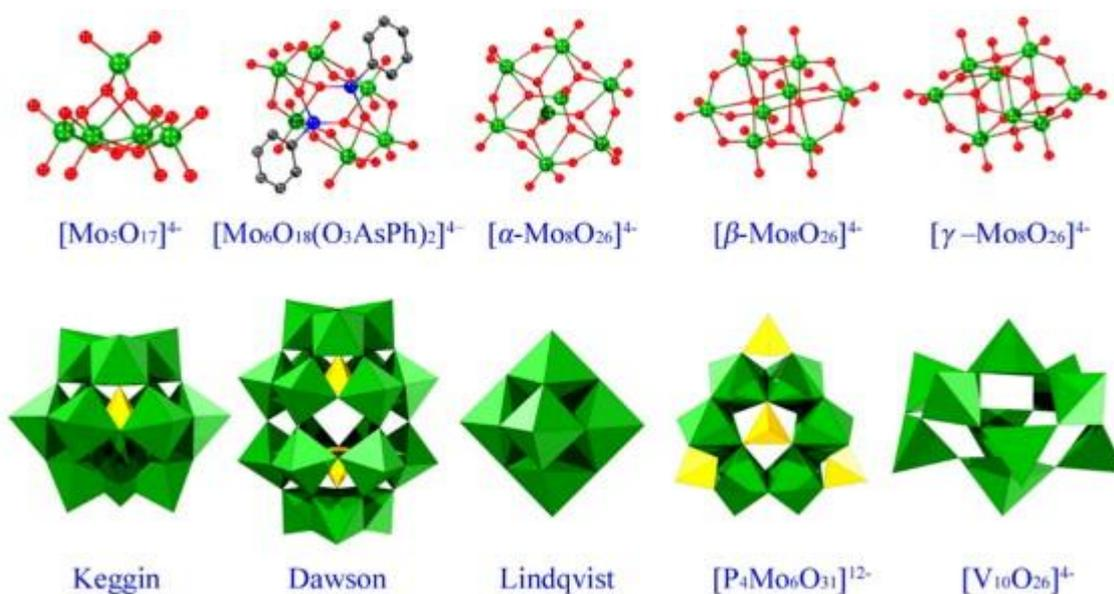
Fig 1; Examples of polyoxometalates.
