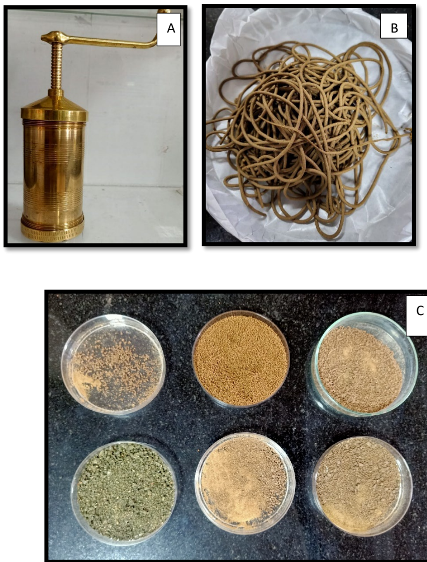
Figure 4: (A) Feed extruder machine (B) Extruded fish feed (C) Feed after crushing into floating micropellets.
