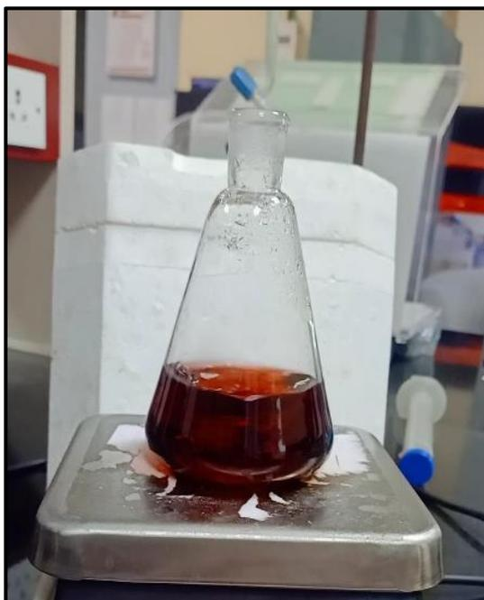
**Figure 4 Red colloidal solution of AuNPs**
