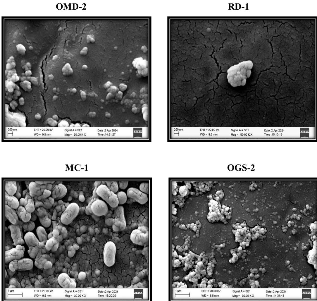
**Fig 4.24: SEM of plastic pieces in MV broth (a) OMD-2 (b) RD-1 (c) MC-1 (d) OGS-2 for 15 days of incubation**
