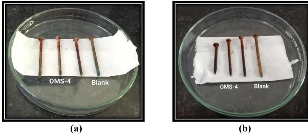
**Fig 4.8: Biofilm formation on nail by OMS-4 isolate (a) 24 h (b) 48 h**
