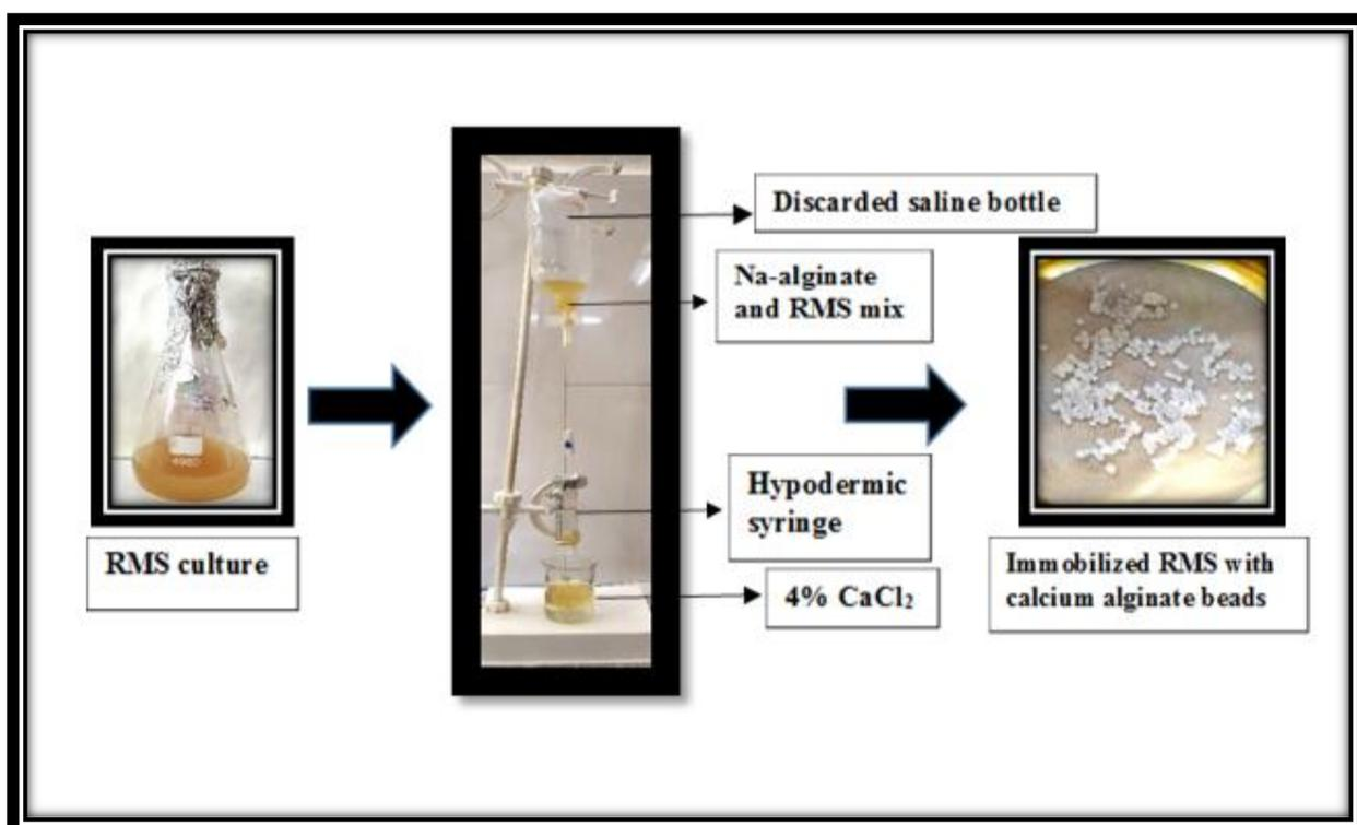
**Fig 3.1: Schematic representation for immobilising RMS within sodium alginate beads using a hypodermic syringe clamped stand and discarded saline bottle.**
