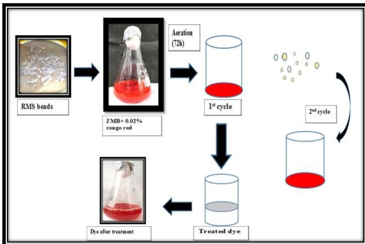
**Fig 3.2: Schematic representation of batch model reactor for treatment of dye.**
