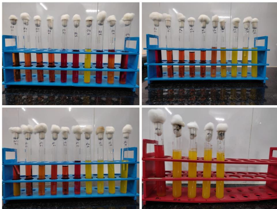
Fig 5: MPN tubes after the incubation period.
