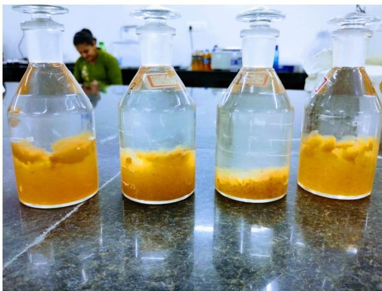
Fig 8: D.O. bottles after fixing the sample with Winkler's A and Winkler's B
