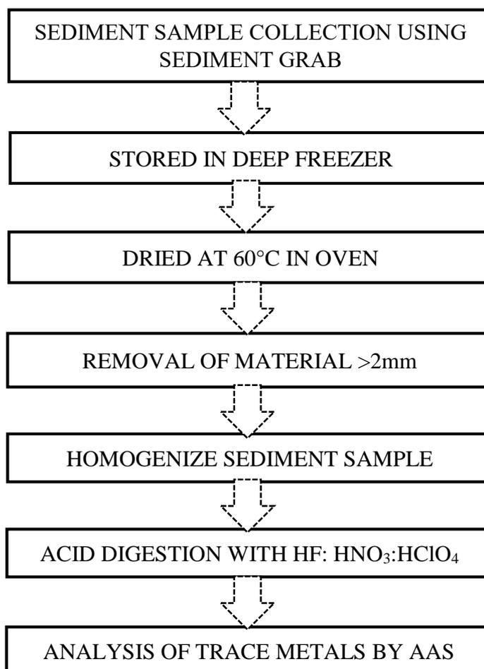
**Fig. 2 – Analytical procedure for estimation of trace metals from sediments.**
