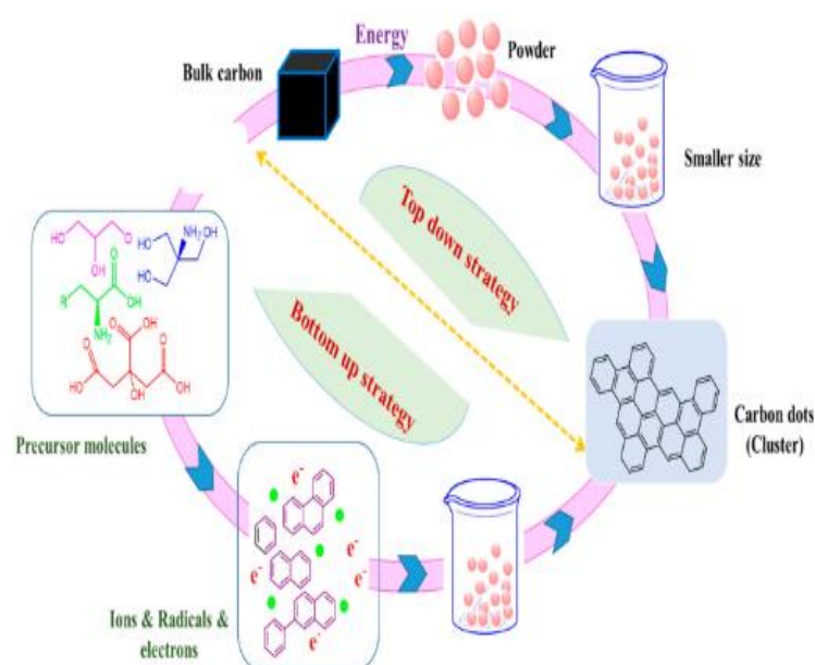
Figure 2. Generation of carbon dots by well-known Top-down and bottom-up approaches.
