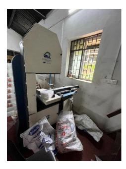
This machine is used for cutting the toilet rolls into its desired sizes.
