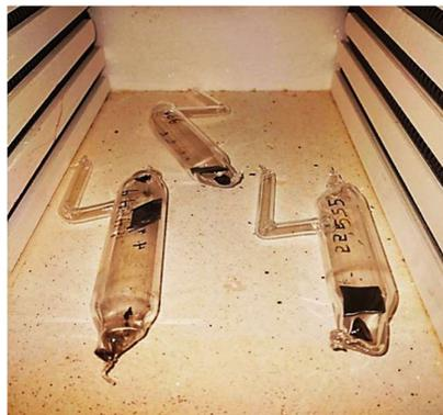
**Fig 2.1.2: Quartz tubes containing samples**
