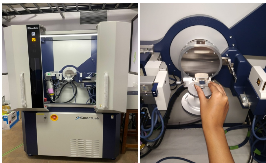
Fig.6. Rigaku XRD machine
