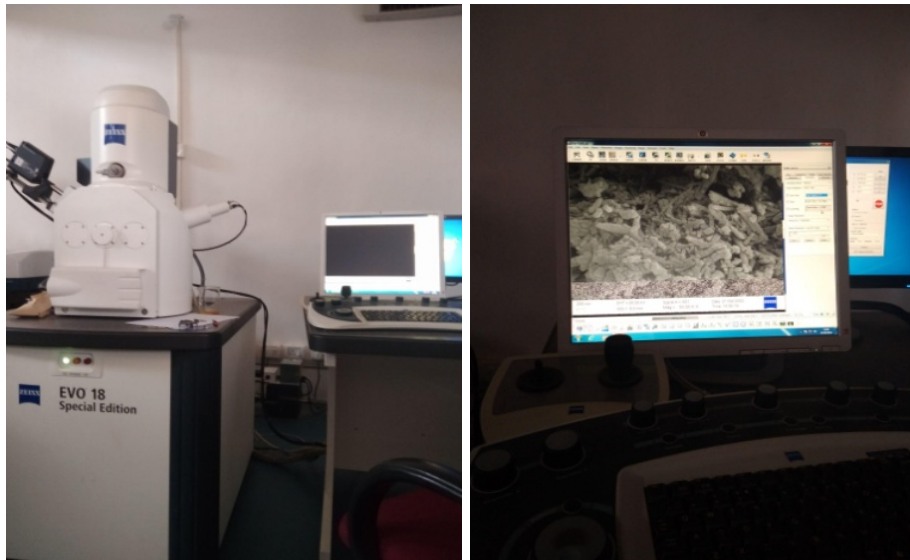
Fig.8. SEM instrument-Zeiss EVO 18 system
