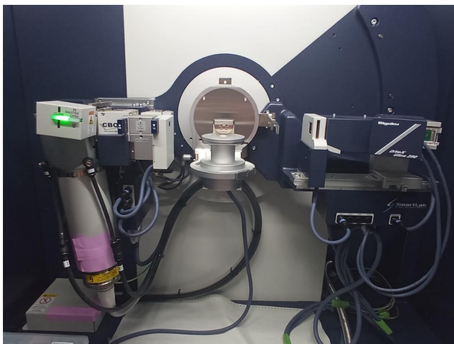
Figure3.4: Rigaku Smart Lab Powder X-ray diffractometer at ULMC of Goa University.
