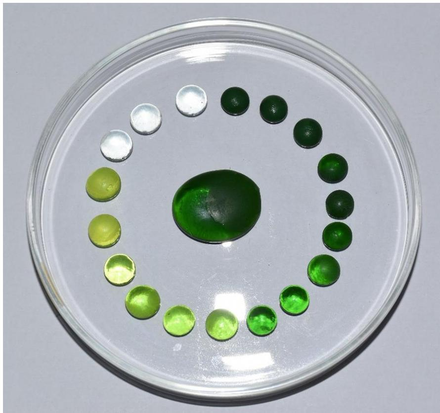
**Figure 17:** Glass beads of various percentages of  $\text{Cr}_2\text{O}_3$
