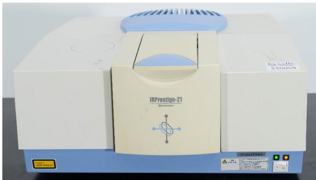
**Figure 10:** Infrared spectrophotometer - Prestige-21
