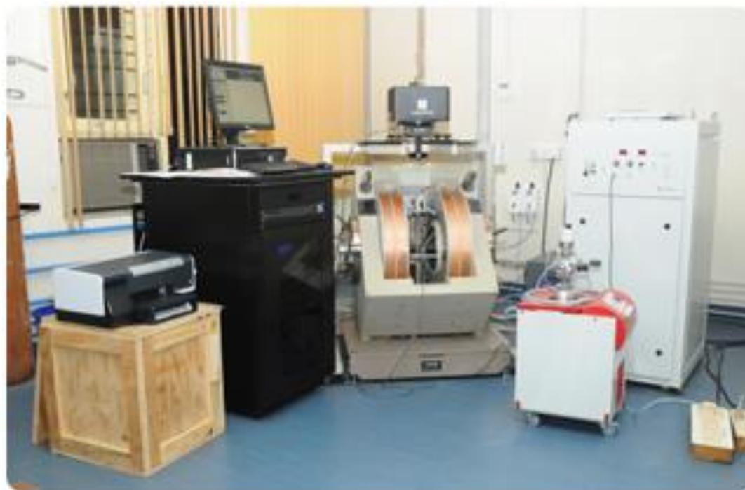
Figure 4.13 - Lakeshore Vibrating sample magnetometer
