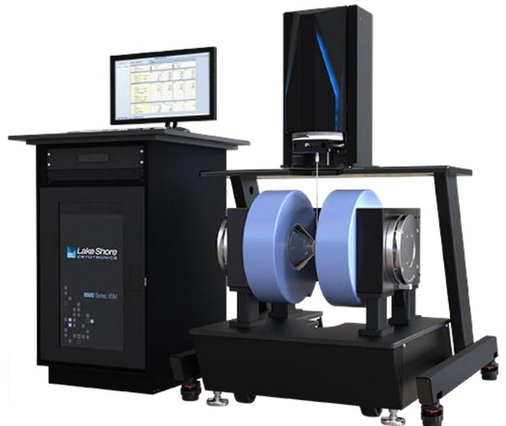
Figure 3.8 - Lakeshore VSM Setup <sup>[15]</sup>
