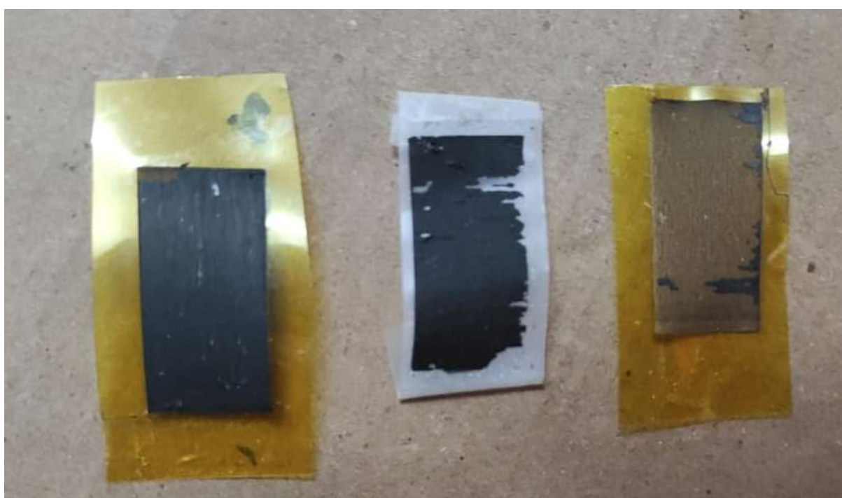
Fig 4.7 Image showing LIG on kapton substrate (left) kapton transferred onto Scotch tape (centre) and Kapton afer removing the LIG (right)
