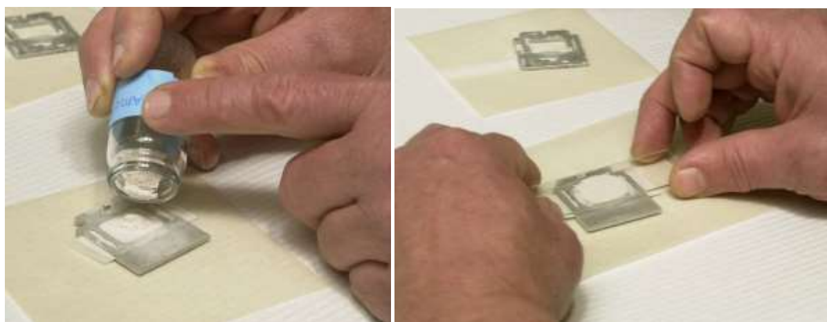
Fig 3.5 Sample preparation for PXRD
