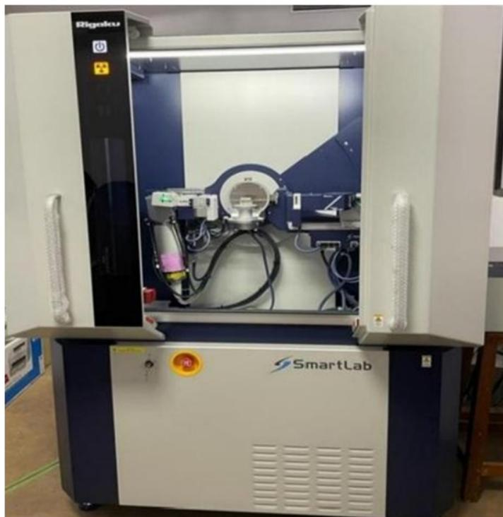
Figure 16: Rigaku Smart Lab Powder X-ray diffractometer at ULMC of Goa University.
