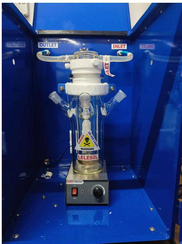
Figure 25: Photochemical Reactor at SPAS, Goa University
