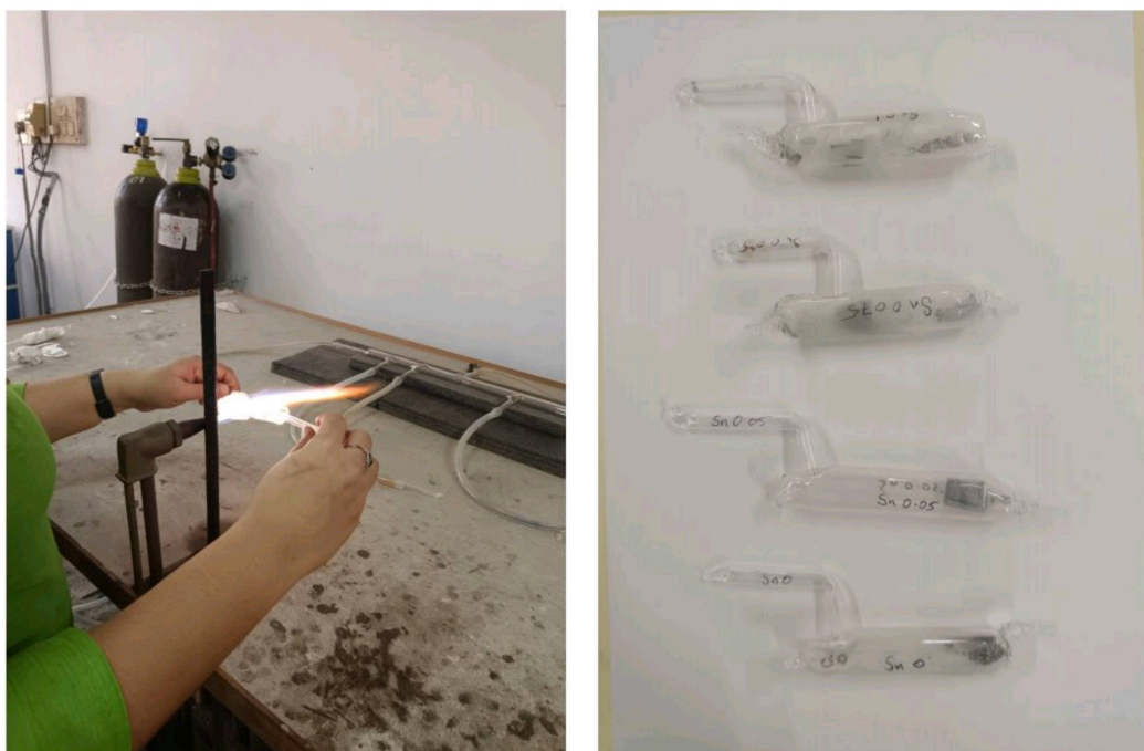
Figure 2.2: Sample sealing procedure and sealed sample before annealing
