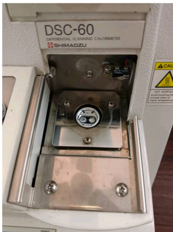
Figure 2.7: Differential Scanning Calorimetry (DSC)- Shimadzu DSC-60
