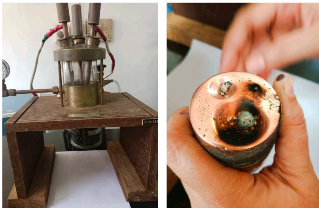
Figure 2.1: Centorr Arc Furnace and sample placed in the crucible of the furnace
