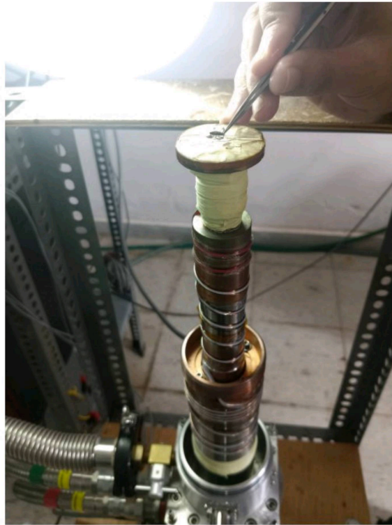
Figure 2.5: Electrical Resistivity Set-up
