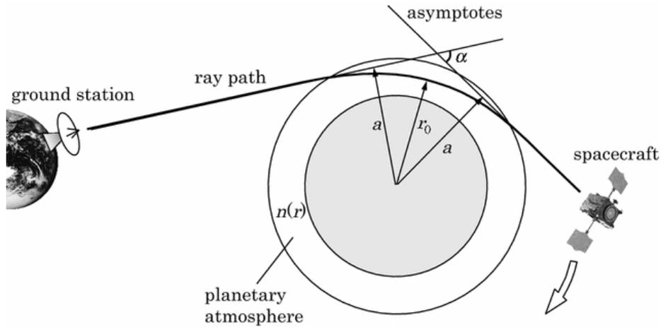
Figure 4.1: Schematic of Radio Occultation Experiment [1]
