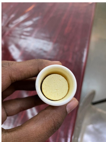
Figure 2.3: Solid g-C 3 N 4 sample obtained using Melamine as the precursor
