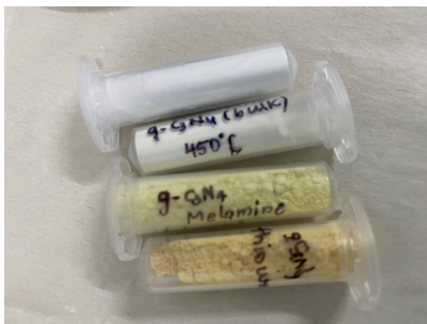
Figure 2.4: Displays solid g\text{-C}_3\text{N}_4 samples synthesized at 450^\circ\text{C} , 550^\circ\text{C} and 650^\circ\text{C} .
