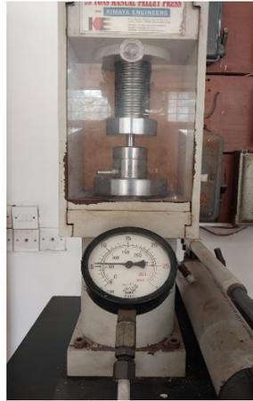
*Figure 31: Set up of a pelletizer.*
