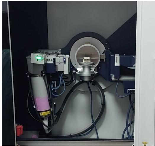
Figure 16: Rigaku Smart Lab X-Ray Diffractometer.
