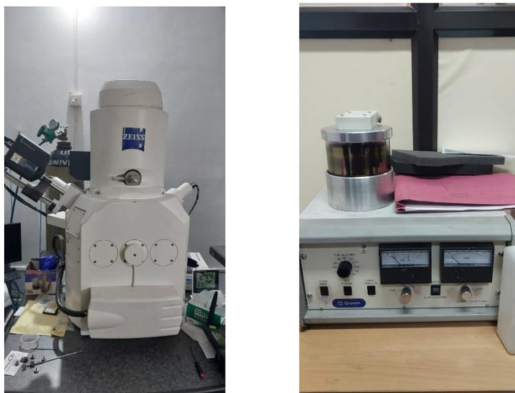
*Figure 26: Carl Zeiss Scanning Electron Microscope and Sputter coater setup.*
