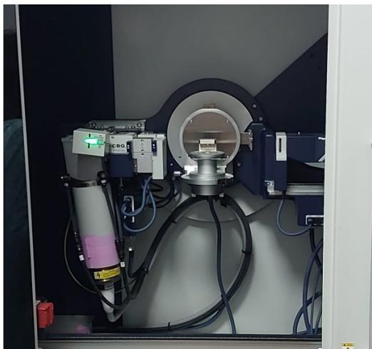
*Figure 23: Rigaku Smart-Lab X-ray Diffractometer*
