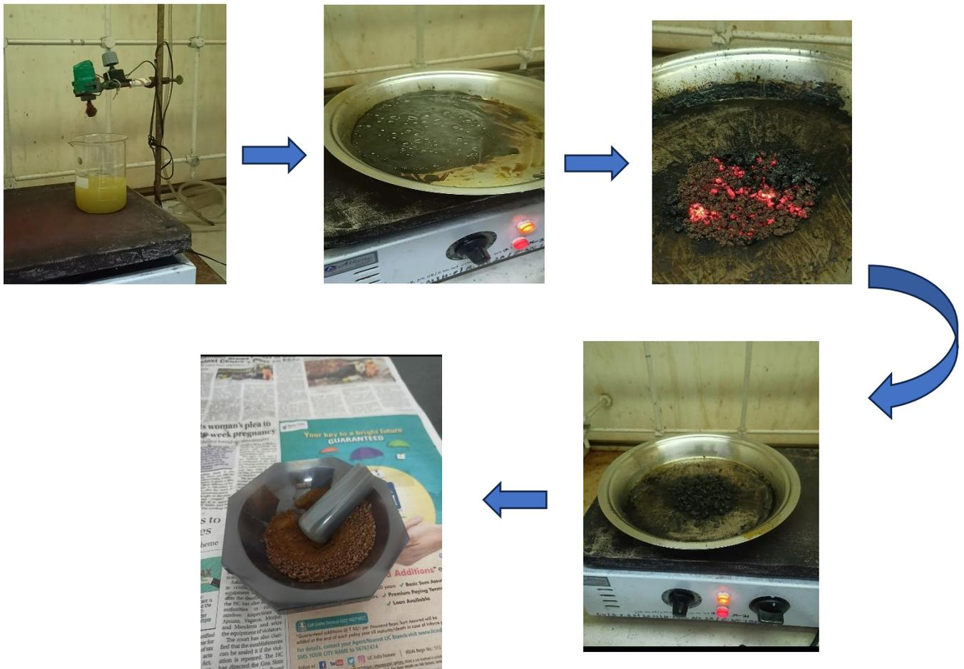
Figure 7:Auto-combustion method
