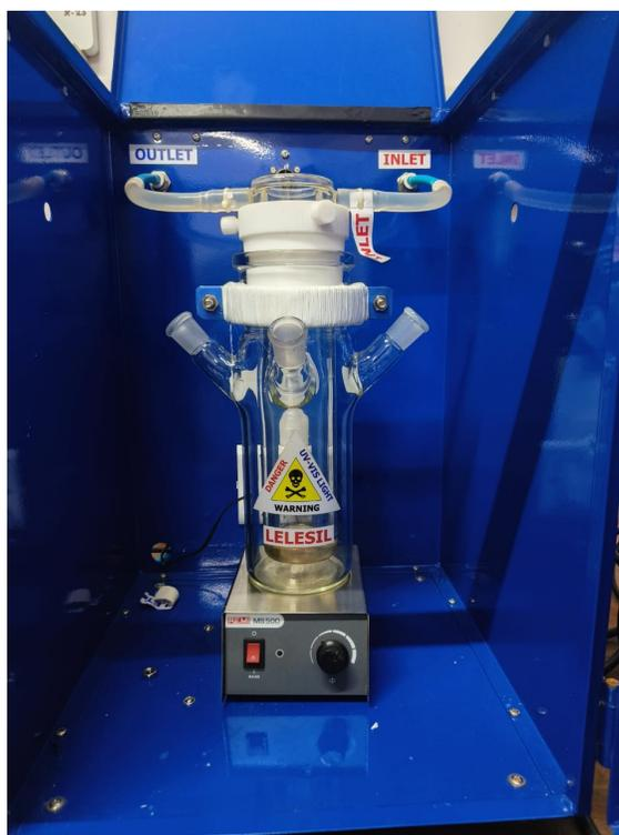
Figure 5.17: Photocatalysis setup at Goa University
