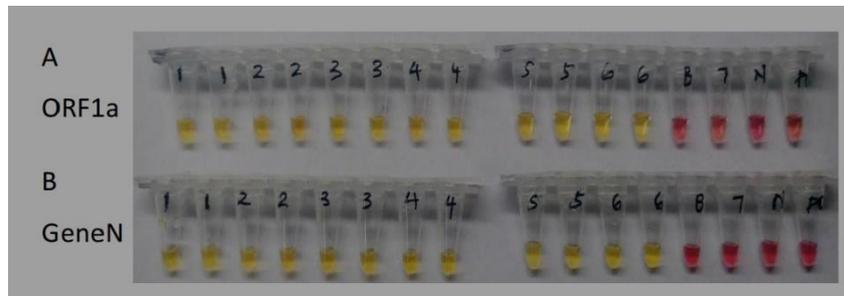
(fig. b). Yellow indicates positive detection after 30 minutes of incubation for sample (1-6) and pink a negative reaction for sample (7) with results compared to negative control (N) <sup>11</sup>
