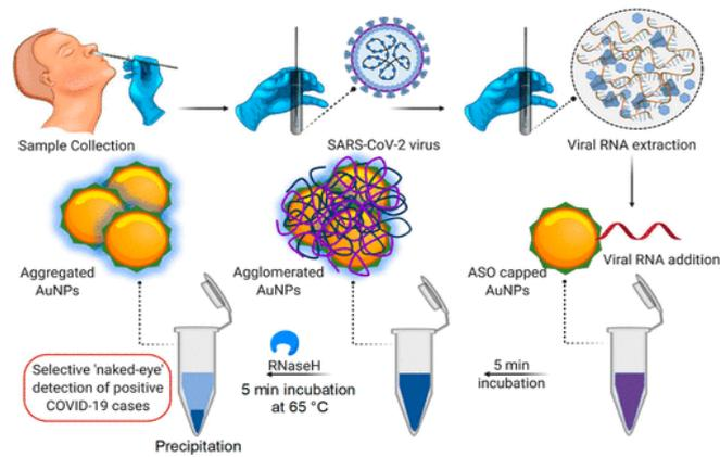
(fig.c) Selective Naked eye detection of SARS-CoV-2 RNA by the suitably designed ASO-capped AuNPs<sup>19</sup>
