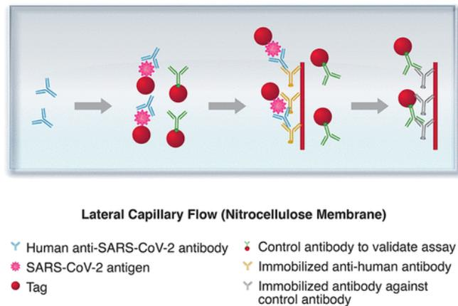
(fig. d). Lateral flow immunoassay for detection of anti-SARS-CoV-2 antibodies<sup>4</sup>
