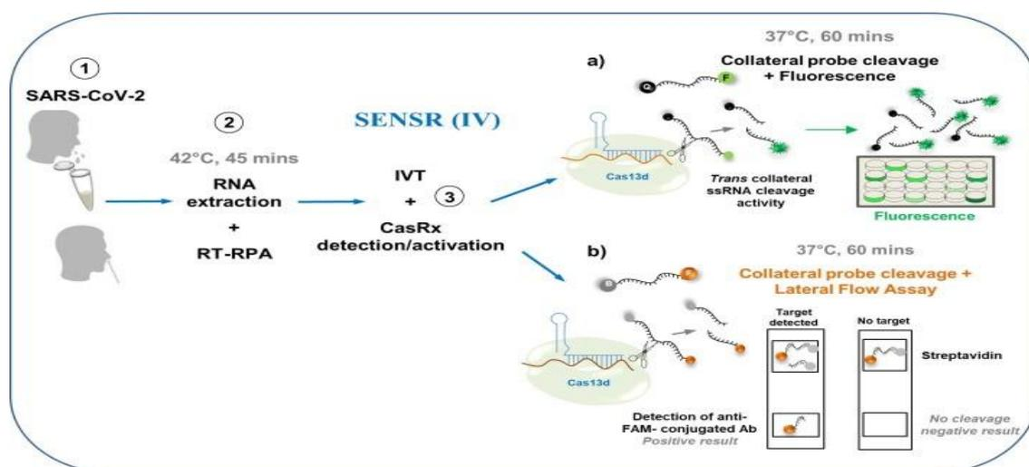
(Scheme 4). Workflow of SENSR based detection of SARS-CoV-2
