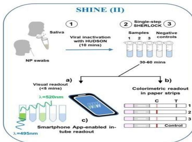
(Scheme 2). Single step SHERLOCK assays using extracted RNA with a fluorescent or colorimetric readout.
