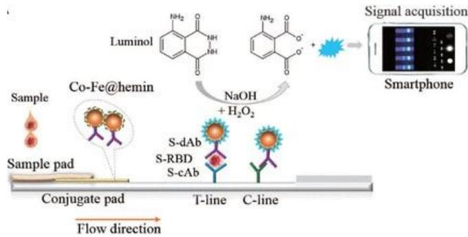
(fig. c). Nanozyme-based chemiluminescence paper test for SARS--CoV-2 S-RBD antigen<sup>30</sup>
