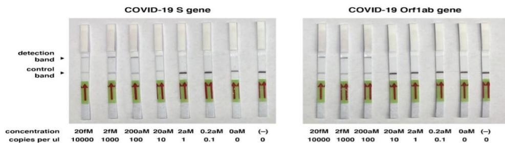
(fig. d). Lateral flow readout for different input concentration.<sup>21</sup>
