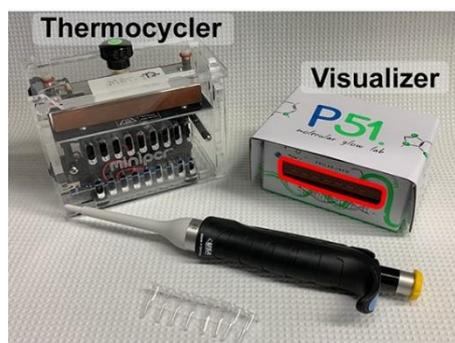
(A)- the miniPCR mini16 thermocycler and P51 molecular fluorescence visualizer used, both of which are portable, can be operated with batteries and have minimal footprint. (B)- Fluorescent visualization of N1, N2, and N3 synthetic targets using P51 visualizer<sup>23</sup>
