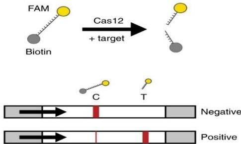
(fig. b). DETECTR coupled with lateral flow readout<sup>19</sup>
