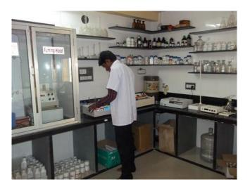
Every hour, water samples are taken from the bottles and numerous tests are carried out. It is first tested for odour, alkanity, chlorine, and calcium, if present. PH METER, TDS (TOTAL DISSLOVE SOLIDS) METER, NEPHLOMETER,
