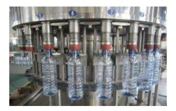
For the purpose of filling, there are three types of filling machines. Bottles of 500ml, 1liter, 250ml are among the sizes that have been filed. When the bottle is first run through JET MACHINES, it is ozonized. This involves integrating and disintegrating the bottle, rinsing it, and then filling the bottles with water.
