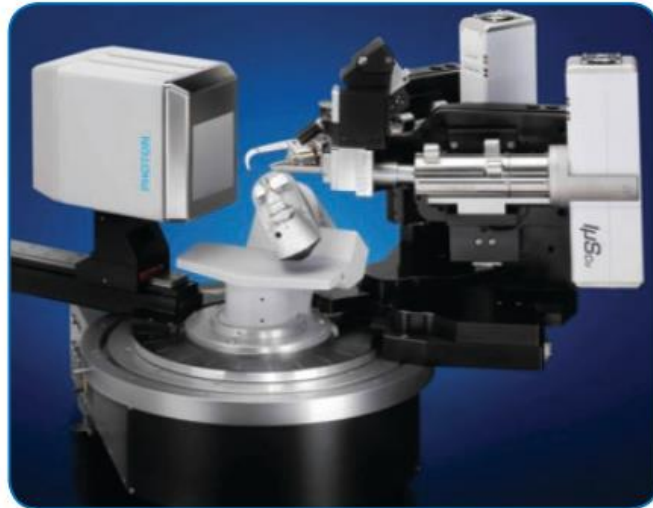
Figure 9. A commercial CMOS-based single-crystal X-ray diffractometer system [10].
