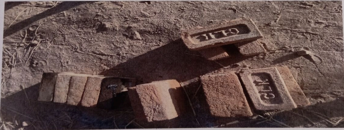
Figure 8: Finished product of brick of this study at Mana village, Raipur district, Chhattisgarh
