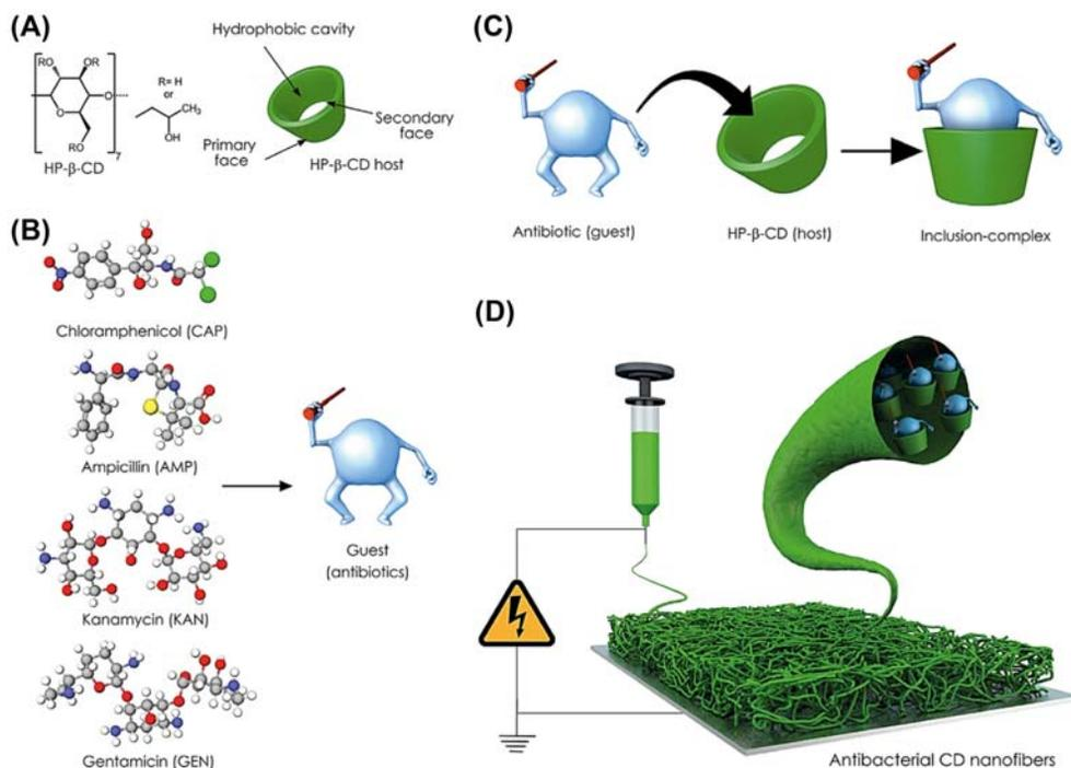
**Figure 18.7** (A) Structure of HP- $\beta$ -CD, (B) high potency antibiotics, (C) molecular models for IC of HP- $\beta$ -CD with antibiotics, (D) diagrammatic electrospinning process. (The copyright permission from F. Topuz, M.E. Kilic, E. Durgun, G. Szekely, *Fast-dissolving antibacterial nanofibers of cyclodextrin/antibiotic inclusion complexes for oral drug delivery*, *J. Colloid Interface Sci.* 585 (2021) 184–194. <https://doi.org/10.1016/j.jcis.2020.11.072>, Elsevier Publisher.)
