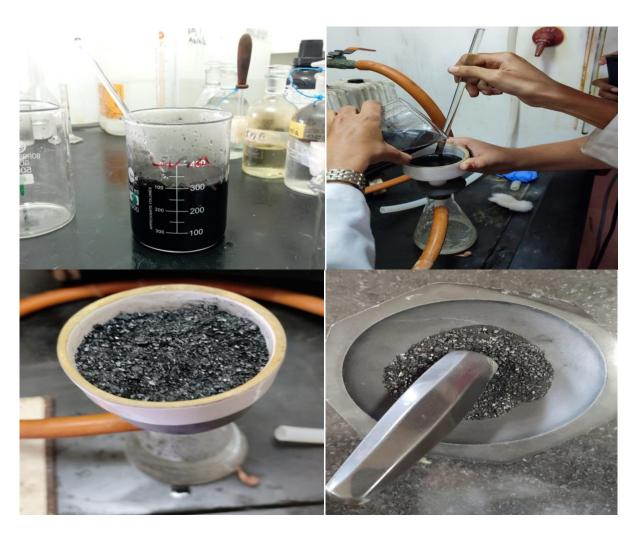
The goal was to use the prepared activated charcoal for use in the incenerator. The harmful/toxic gases like furan and dioxins were to be adsorbed onto the charcoal bed and further analyse its efficiency. Due to time constraints we couldn't go on further with the experimental work
