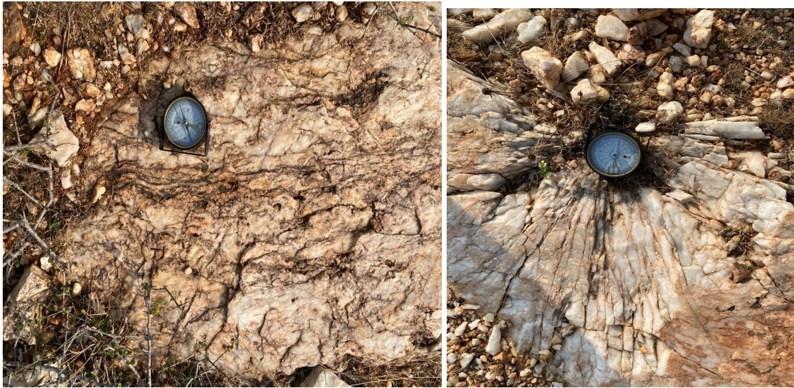
Fig 26;A) Tensional and extensional joints. B) Radial joints.
