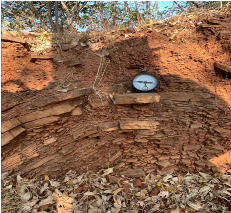
Fig 25; Folding in Phyllite. (Clinometer as a scale)
