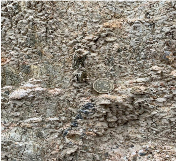
Fig 9 ; Caliche deposits,a coin as a scale.
