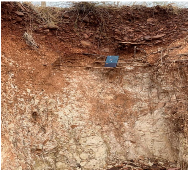
Fig 7:cross section of A thick layer of conglomerate,20cm notebook as a reference.
