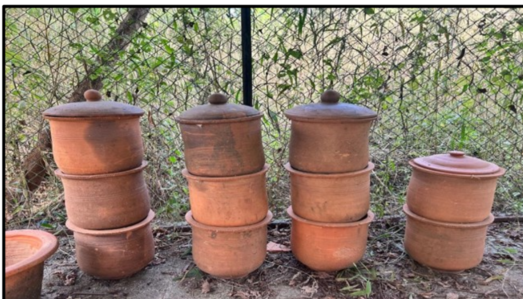
Fig. 7.9. Compost acceleration process at Pilot Scale using Khamba assembly
